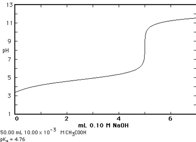
Figure 1. Titration of a weak acid with strong base, NaOH.
