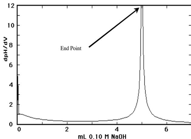
Figure 2. Derivative plot of the acetic acid titration shown in Figure 1.
