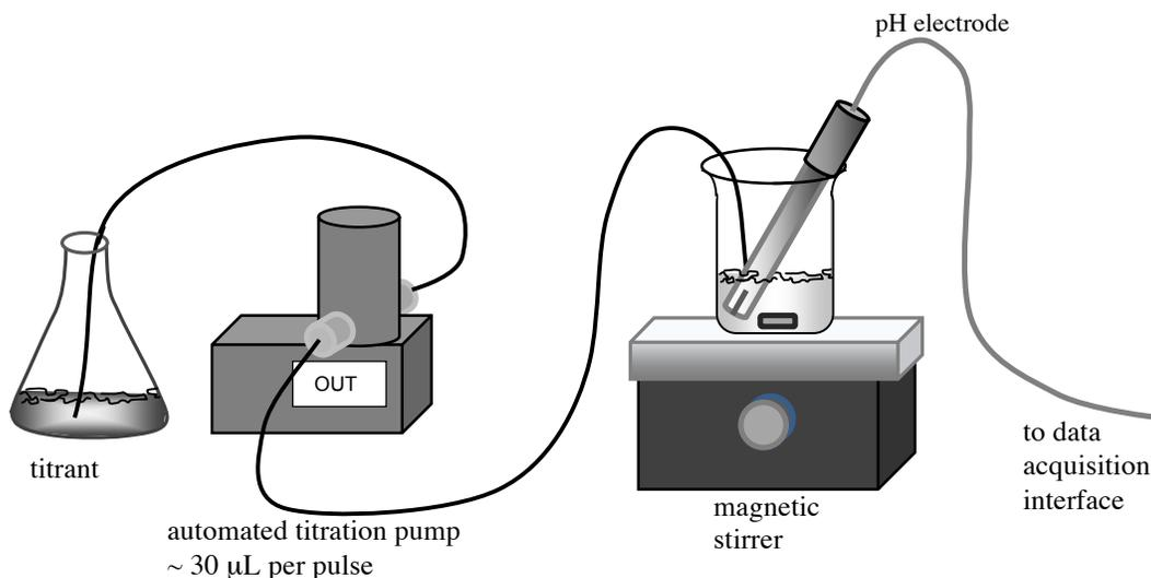
Figure 4. The automated titration system is based on a computer controlled titration pump. The progress of the titration is monitored using a pH electrode.
