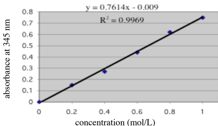
Figure 1. A typical absorbance vs. concentration standard curve based on Beer's Law. This particular curve is most reliable for absorbance values between 0 and 0.8. The concentration for a solution can be determined by measuring its absorbance and then substituting the absorbance value as  $y$  in the equation for the standard curve and solving for  $x$ .
