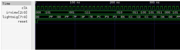
For Task 6, we had to set the code up so that it would work with a physical circuit. This was just a matter of setting up the pins, then changing the clock, for our purposes, to go 32 million times slower than the actual internal clock so we could see our results. A video of me testing my circuit is below. As we can see, the board cycles through all of the instructions we gave it in the lightrom, represented by the red LEDs, and the output is represented by the green LEDs.
