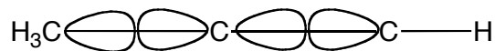
C–C \sigma -bonding in propyne ("small" lobes of the orbitals are not shown)
